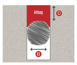
**B** = Joint width **D** = Joint depth
